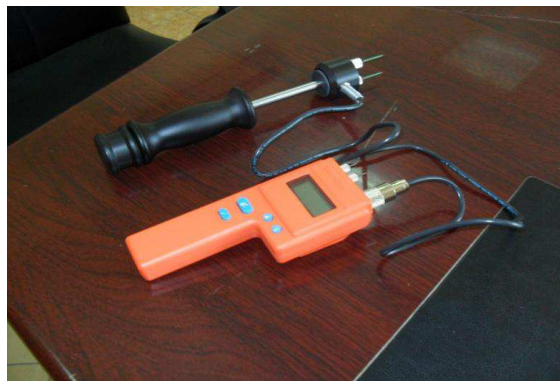
Figure 2: Photograph of Instrument Model RC-2 for Measuring MC of Palm Trees Waste
